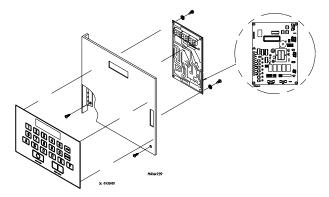
Remove the screws securing the computer to the sheet metal control panel. Remove the board by pulling the other two corners off the clinch studs.
